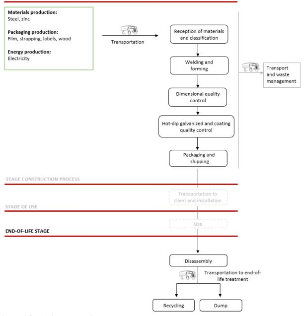
Image 1 Production process diagram.
