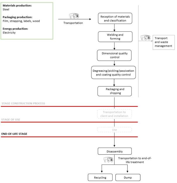
Image 1 Production process diagram.
