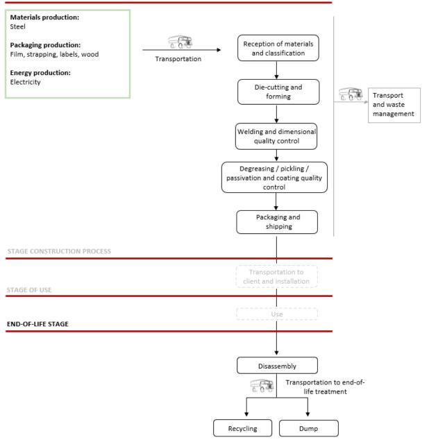
Image 1 Production process diagram.
