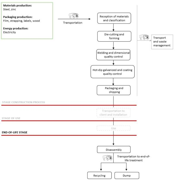
Image 1 Production process diagram.
