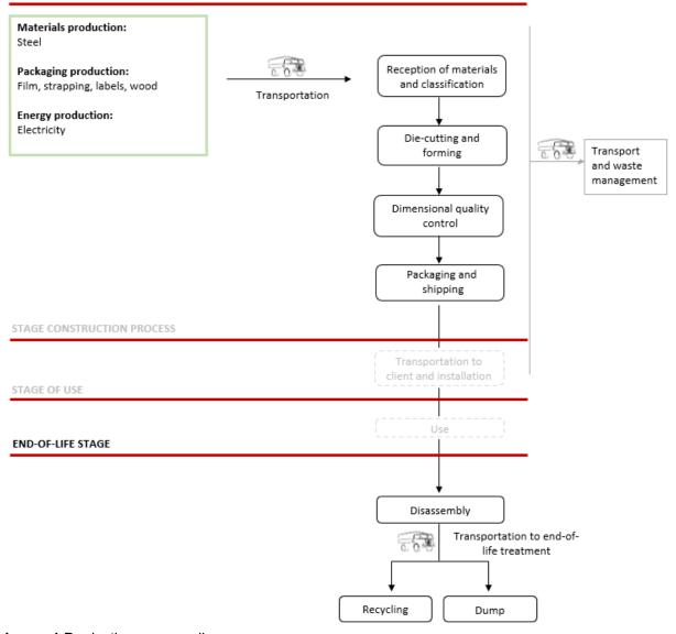
Image 1 Production process diagram.
