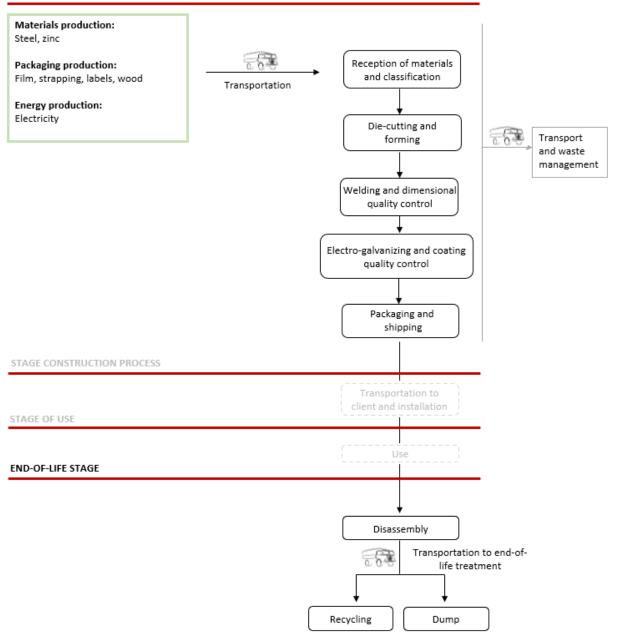
Image 1 Production process diagram.
